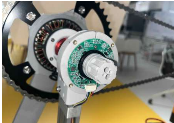
Figure 2-19: Encoder mounted on the test stand
