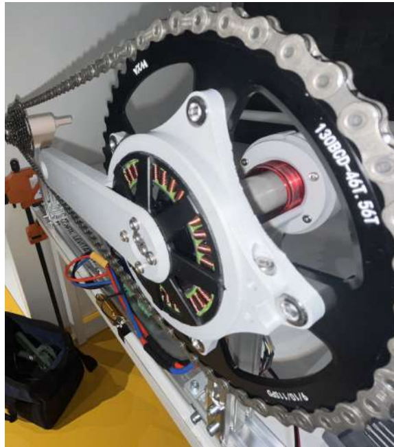
Figure 2-5: Motor integrated into the chainring. The copper wire is wound on the stator of the motor.
