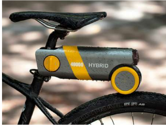
Figure 1-3: Example of a friction-driven motor. The power is transmitted through friction between the small wheel and the bicycle rear wheel.
