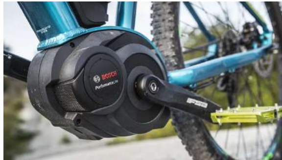
Figure 1-1: Example of a mid-drive motor. The motor and gearbox are located on the bottom bracket of a proprietary bike frame.
